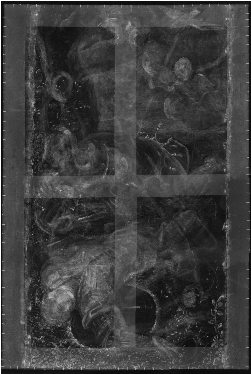
Figure 22. Tancred Baptizing Clorinda , x-radiography image captured with Pantak-Seifert x-ray tube at the following parameters: 25kV, 3 \mu A, 45 seconds, 40" distance from tube. Captured in 20 sections, composite image created in Adobe Photoshop CS6.
