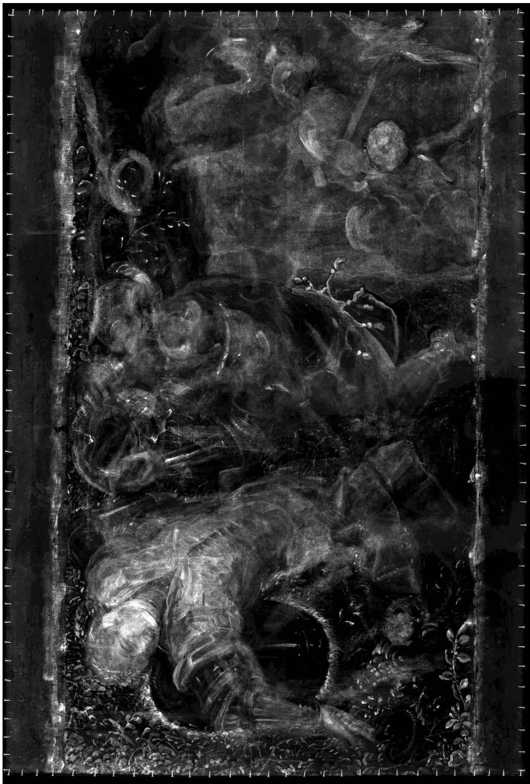
Figure 23. Tancred Baptizing Clorinda , x-radiography image captured with Pantak-Seifert x-ray tube at the following parameters: 25kV, 3 \mu A, 45 seconds, 40" distance from tube. Captured in 20 sections, composite image created in Adobe Photoshop CS6. Image digitally altered to minimize the appearance of stretcher bars and enhance the contrast.
